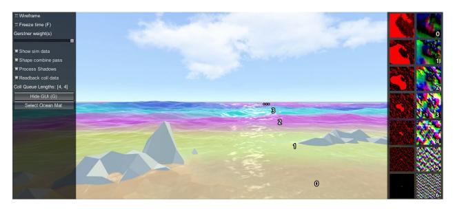
In the above screenshot the foam data is also visualised (red textures), and the scale of each LOD is clearly visible by looking at the data contained within. In the rendering each LOD is given a false colour which shows how the LODs are arranged around the viewer and how they are scaled. Notice also the smooth blend between LODs - LOD data is always interpolated using this blend factor so that there are never pops are hard edges between different resolutions.
