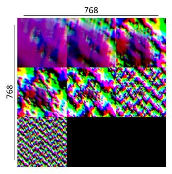
A final feature of the LOD system is that the LODs change scale with the viewpoint. From an elevated perspective, horizontal range is more important than fine wave details, and the opposite is true when near the surface. The *Ocean-Renderer* has min and max scale settings to set limits on this dynamic range.
