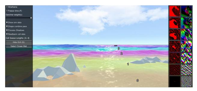
In the above screenshot the foam data is also visualised (red textures), and the scale of each LOD is clearly visible by looking at the data contained within. In the rendering each LOD is given a false colour which shows how the LODs are arranged around the viewer and how they are scaled. Notice also the smooth blend between LODs - LOD data is always interpolated using this blend factor so that there are never pops are hard edges between different resolutions.
